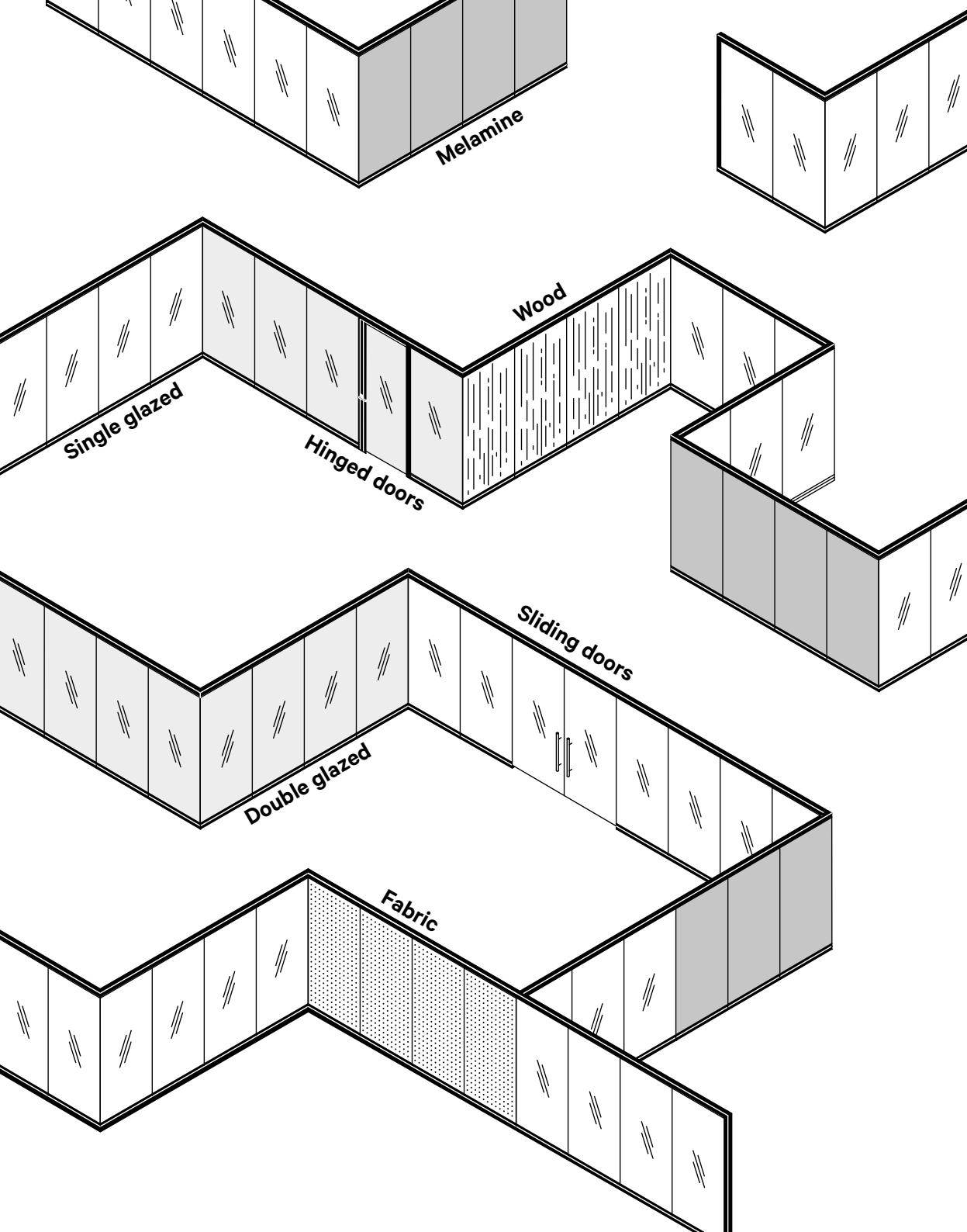
A partition wall whose single technological profile, with a total thickness of only 80 mm, is able to accommodate a wide variety of materials in a seamless aesthetic continuity - glass, wood, metal, fabric, shelf and wall unit fittings, integrated wiring, and monitors - all along the same elevation. In addition to partitions for space division, cladding versions are also available.
